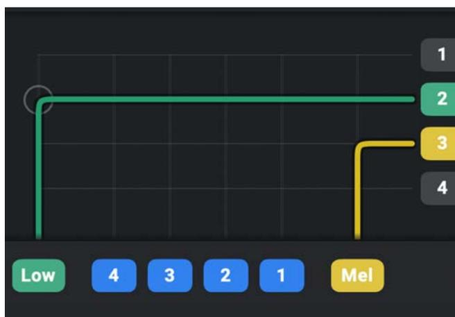
The routing matrix allows you to distribute the voices and ranges across the output ports and modify the notes and controllers that are coming through.
